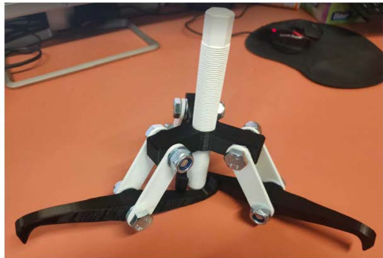
Figure 7 3D printing of a bearing puller
