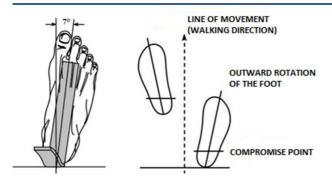
Figure 2 Effect of 7 ° outward rotation of the spring on the walk [2]
