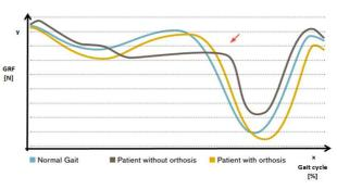
Figure 4 Illustration of increased knee dynamics when walking with AFO[2]
