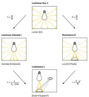
Figure 2 Basic parameters used in lighting [17]
