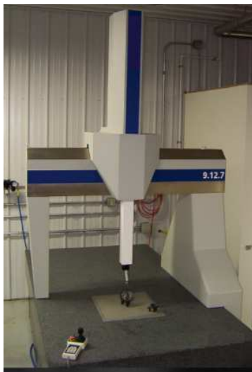
Figure 1 A coordinate measuring machine with rigid perpendicular arms [2]
