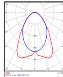
Total lamp luminous flux: 44400 lm, Total luminaire luminous flux: 36330 lm, Total Load: 648.0 W, Light yield: 56.1 lm/W
